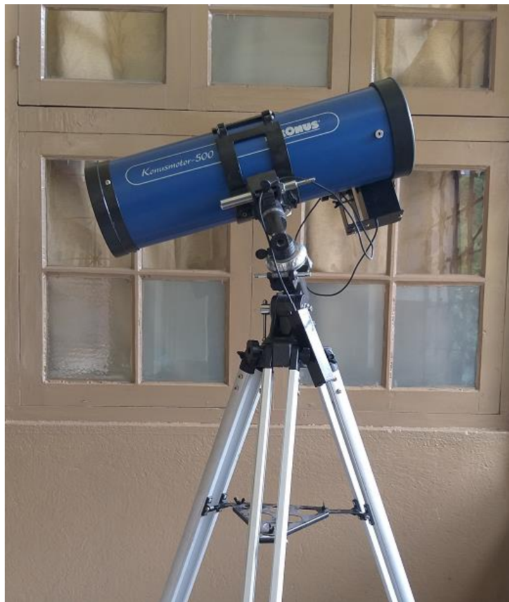
A 4.5 inch Konusmotor – 500, Newtonian Reflecting telescope
